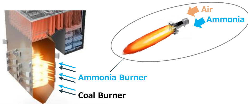
Ammonia Burner (Image only)
