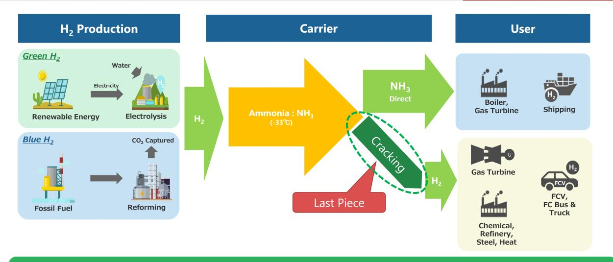
Ammonia cracking technology is the last remaining piece of development. Cracking technology can deliver carbon neutral energy to various users. "Research and development of large-scale external thermal ammonia decomposition hydrogen production technology" project funded by NEDO
